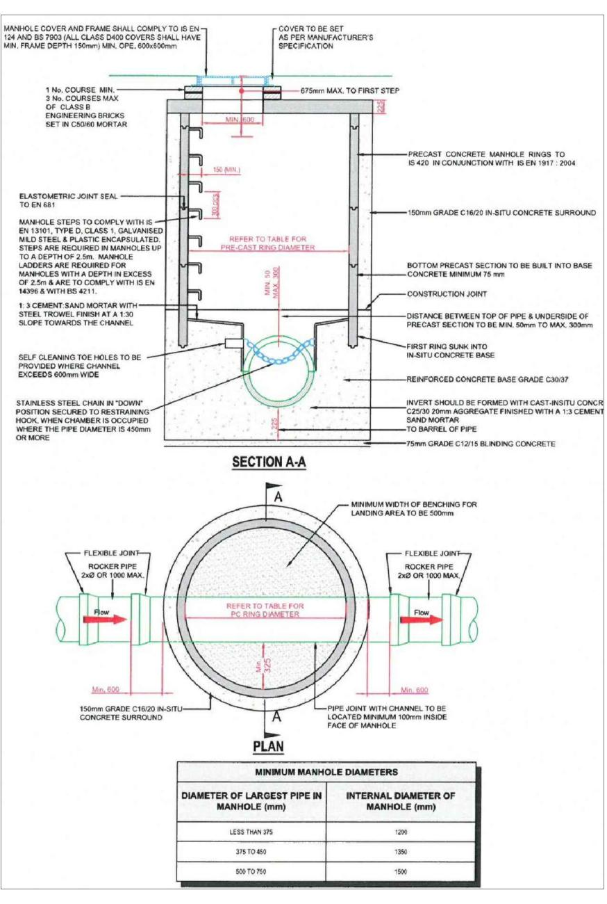
TYPICAL MANHOLE DETAILS (scale 1:25)
